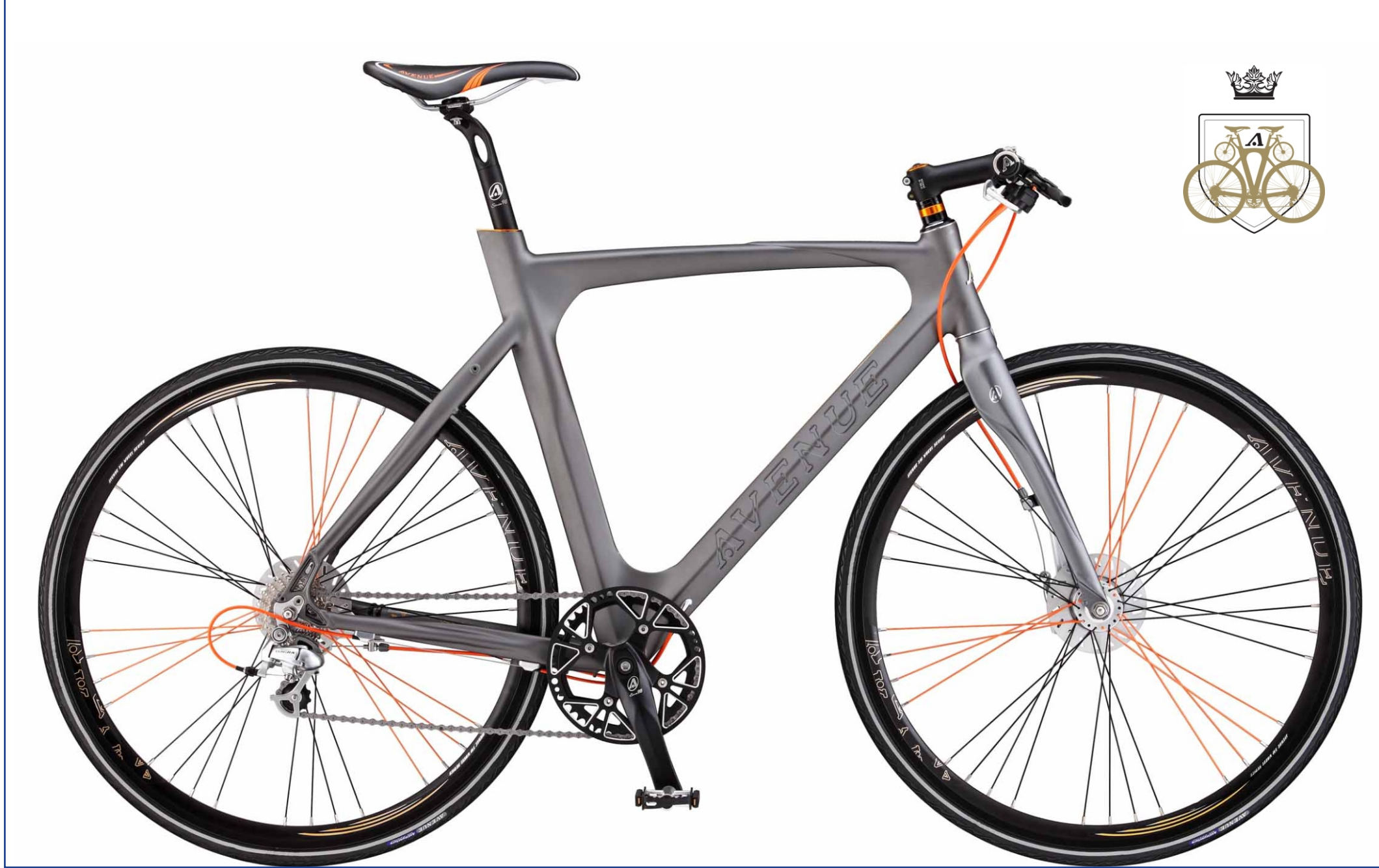
Avenue Airbase magicgrey mat. Shimano Tiagra 9 speed. Shimano IM-55 Rollerbrakes. Exclusive Alloy 7005 w/Carbon shell.
