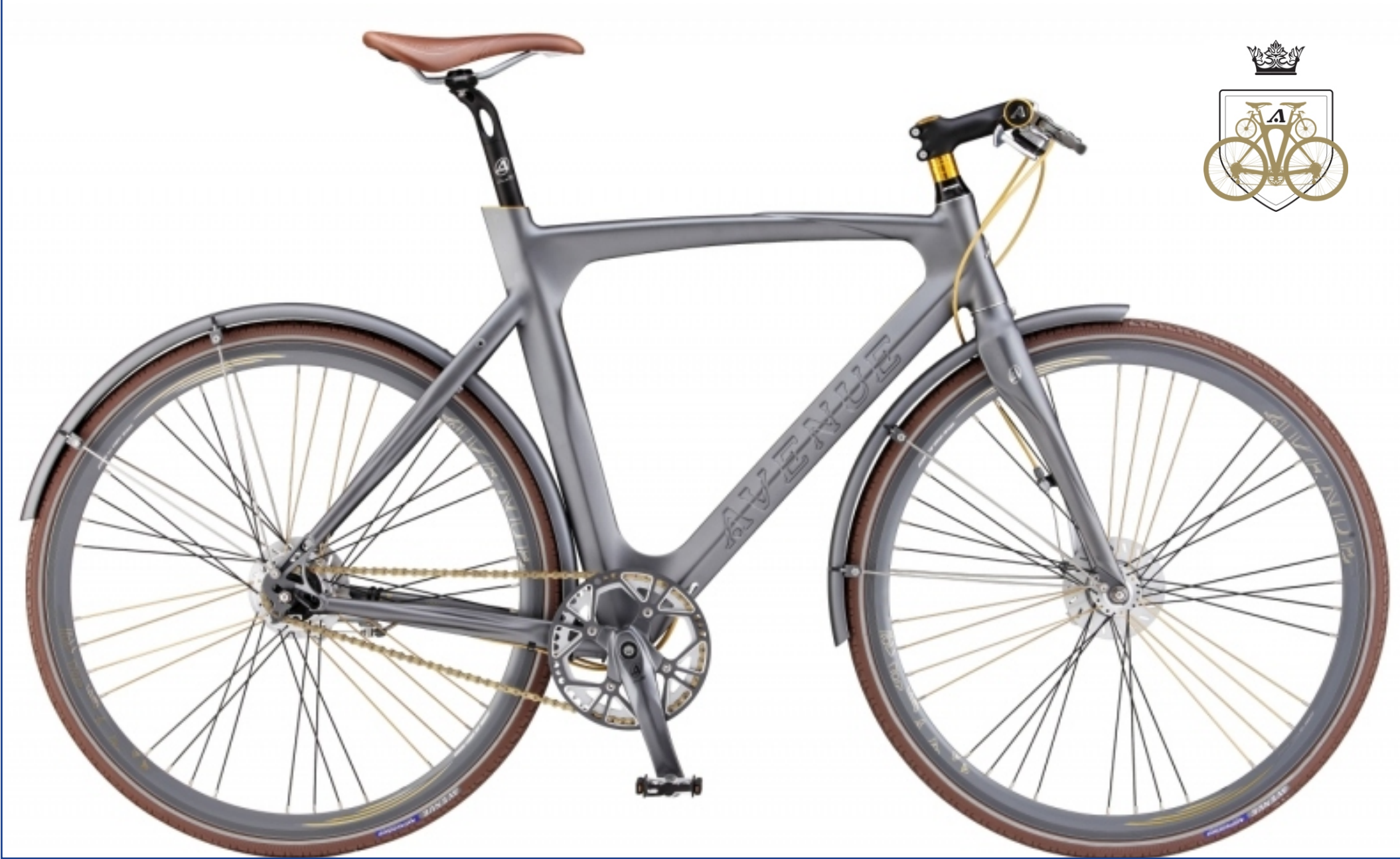
Avenue Broadway Premium. Shimano Nexus 7 speed. Shimano IM-55 Rollerbrakes. Exclusive Alloy 7005 w/Carbon shell.
